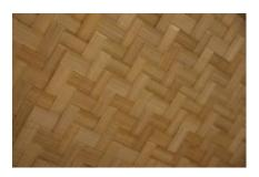
Bamboo Matboards find a wide range of applications from panelling and roofing to interleaving with wood and veneers to create Bamboo veneer. Matboards in India are available at present at anywhere between Rs 27-Rs 65 depending on thickness (indiabambooallinall.org)
